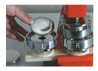
2. Place the shell part of the pin casing onto the left hand mold.
