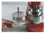
3. Place the cut image, followed by the mylar cover, on top of the shell.
