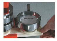
4. Push the mold set to the right and align with the press.
