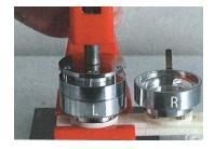
7. Push the mold set to the left and align with the press.
